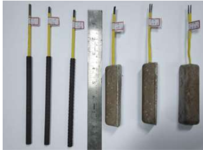
Figure 5.4: Steel and anode samples used for obtaining input parameters
