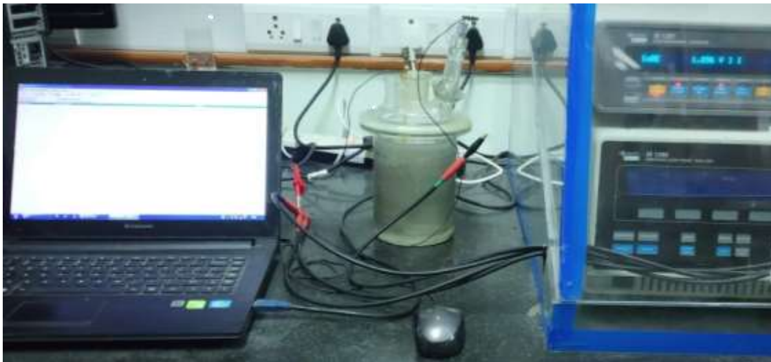
(a) Photograph showing the potentiodynamic test setup
