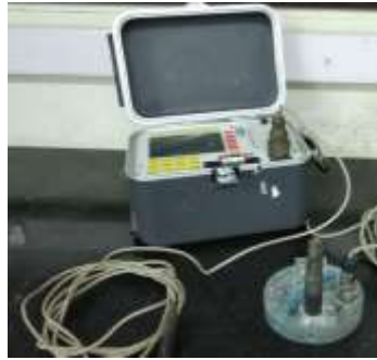
(b) Corrosion rate meter and sensors (Gecor 8™)
