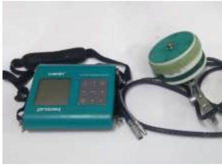
(a) Half-cell potential meter and reference electrode (Canin +)
