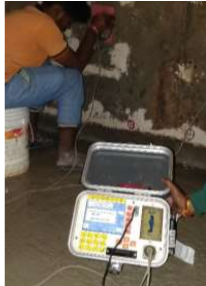
Retaining wall 3 – result displayed 'Well protected'
