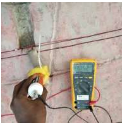
(g) Half-cell potential of the anodes was measured using a Cu/CuSO 4 reference electrode
